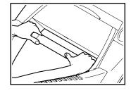
the Heart Rate indicator beside the Calories/Fat Cals./Heart Rate display will light, two or three dashes (---) will appear, and then your heart rate will be shown. For the most accurate heart rate reading, continue to hold the contacts for about 15 seconds.
